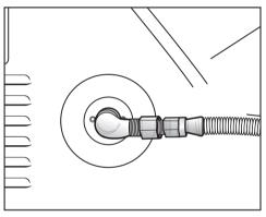
Using two adjustable wrenches tighten the flexible gas line connection.
